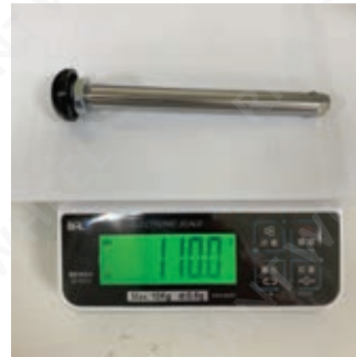
Standard Quick Release - 12.7mm x 4.5" 110.0 g
